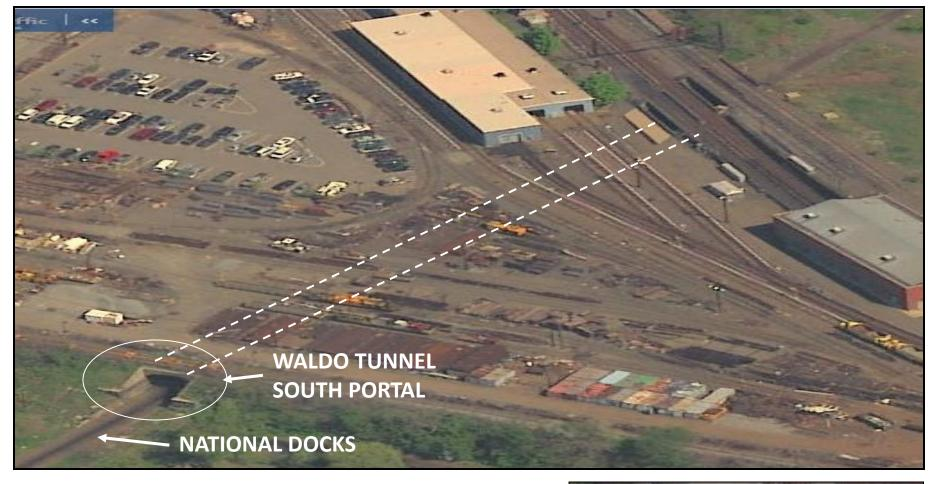
36' FEET OF EXISTING TUNNEL ROOF TO BE REMOVED AND SOUTH PORTAL RECONSTRUCTED
